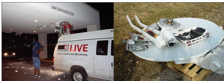
Figure B.5 Clearance accidents occur much more often than any other type of ENG/SNG incidents. Although these mishaps can also cause a threat to life, they most often cause property damage, and damage to one's career. The ENG truck on the left had its mast down, but that was still not low enough to clear this 9'6" hotel canopy. ENG/SNG operators need to know their "on-the-road" clearance. The right photo shows a KU dish that got sheared off a SNG truck when that truck took off with the dish still up.
