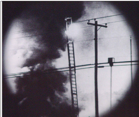
Figure B.1 This photo, from a government safety manual, demonstrates what happens when an aluminum fire ladder touches a high voltage power line, most of which are not insulated. ENG microwave masts have the same conductive characteristics as this ladder.
